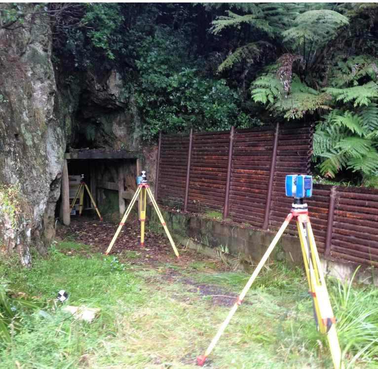
Laser scanning of portal area for vent lock design
