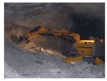
Figure 7 - A Brokk 400D being used in underground narrow vein operations
