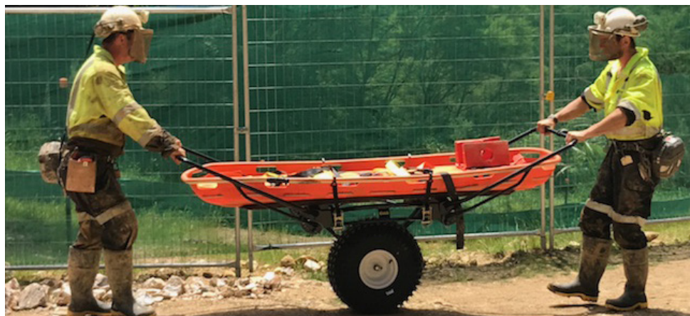
Figure 1 - Team members demonstrating the mono wheel stretcher carrier purchased for underground rescue.
