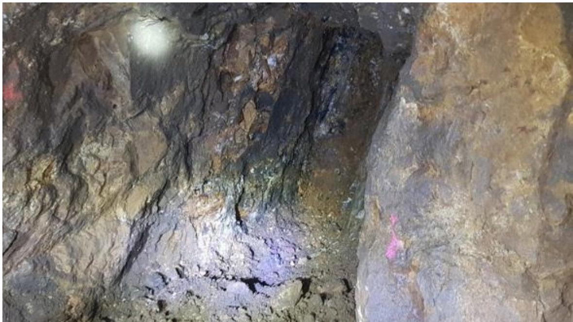
Figure 3 - the face of the Mystery Drive showing the extension of the vein before sidewall waste is removed
