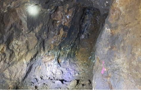
The face of the Mystery Drive showing the extension of the vein before sidewall waste is removed
