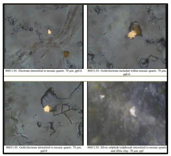
Photomicrographs of gold and electrum plus silver sulphide interstitial with mosaic quartz from the Tafuse Prospect. (Source Applied Petrological Services and Research report to Canterbury Resources)
